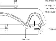
•A sag on the cover tends to arises as the pad is compressed by pressing.
